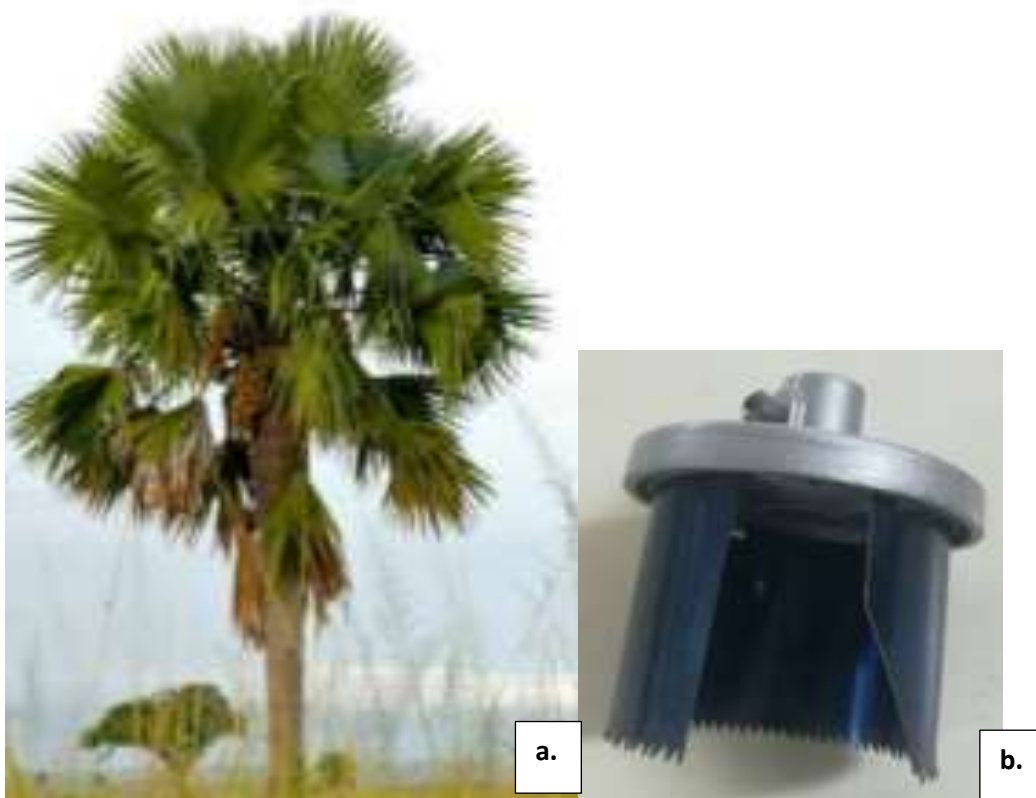
Figure 1: Borassus wood and the coring tool for cutting the sample
